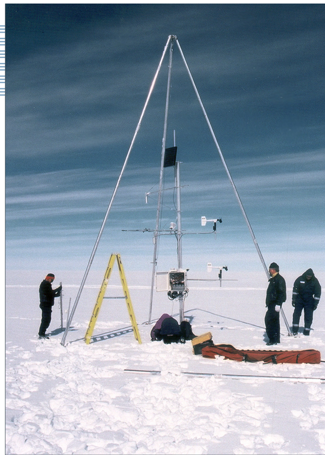
A weather station begins to lean with recent snowmelt. Researchers rode snow-mobiles to steam-drill a new 6-meter (20-foot) hole and secure the station. Credit: John Maurer
